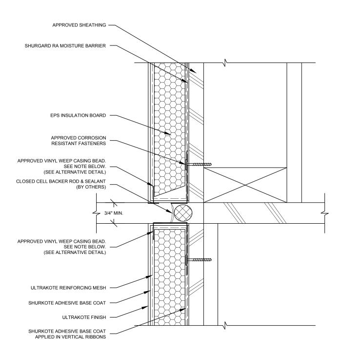
NOTE: MAINTAIN 1 SPACE BETWEEN BEVELED INSULATION AND CASING BEAD
